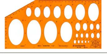
Ellipse Template 4 Angles Ellipse Template, 4 projection angles  $25^{\circ}$ (1:2,38) - 17 Ellip. 4-35 mm, $35^{\circ}16'(1:1,7)$ Isometric - 16 Ellip. 4-32 mm, $45^{\circ}(1:1,4)$ - 15 Ellip. 5-32 mm,  $60^{\circ}(1:1,14)$  - 14 Ellip. 5-30 mm TEMPLATE DIMENSIONS: 260 x 125 x 1.0 mm
